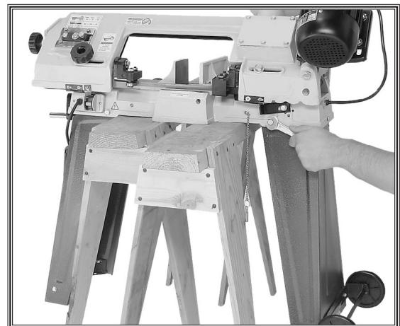
Figure 11. Attaching leg assemblies.
